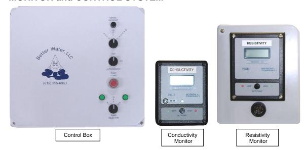
The **Control Box** is a chemical resistant box which contains the electronic components needed to operate the Post-Treatment Rack. Its front panel contains the following: Fuse, Pump Mode Switch, Pump Auto Reboot Switch, Pump Start Button, and the Pump Selector Switch and Indicator Lights. It also houses a **Variable Frequency Drive (VFD)**, to provide maximum pump efficiency to the Repressurization Pump(s).
