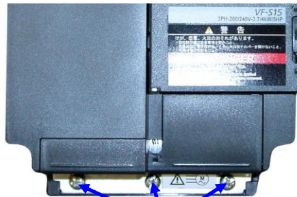
New Model VFD Three grounding posts
